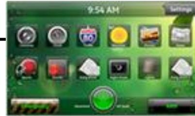
1. Z-Wave widget: light turned on. Command passed to Gateway.
